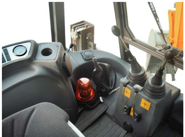
RC3 - Mechanically operated control levers (gear pump)
