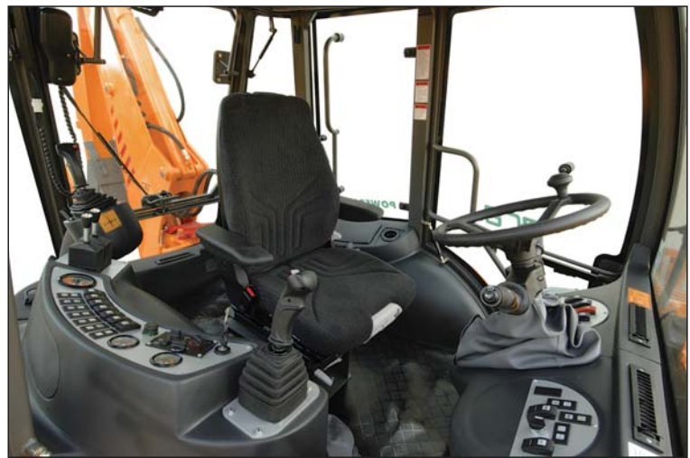
RC5/RC8 - Hydraulic operated JOYSTICK controls enables the operator to have smooth control and get precise movements (RC5: piston pump - RC8: gear pump)
